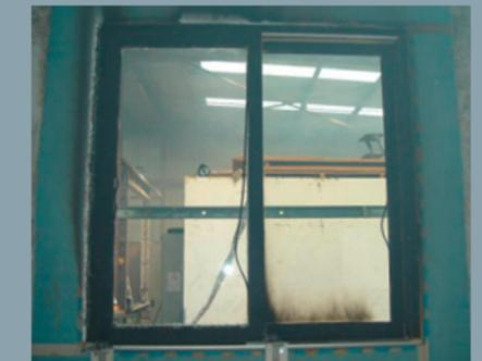
Exposed (Outer) face of a Kömmerling PremiDoor after a BAL 40 AS 1530.8.1 Bushfire Resistance Test
