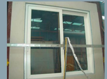
Unexposed (Inner) face of a Kömmerling PremiDoor after a BAL 40 AS 1530.8.1 Bushfire Resistance Test
