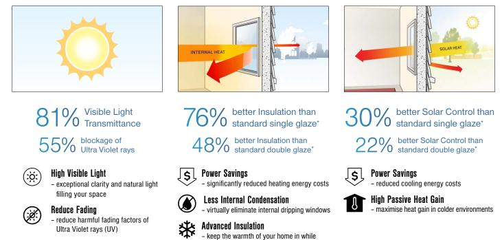
\*Note: Data using centre of glass performance in NFRC standards and using 4mm clear float single glaze, 4/12/4 clear float double glazed unit with air gap and 4/12/4 Insulglass LowE Plus<sup>®</sup> double glazed unit with argon gas and coating to surface #3.
